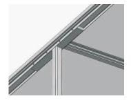
Image shows gutter channel fitted.
