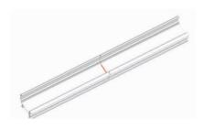
10. Apply a generous amount around the edges of the flat plates inside the gutter and ensure all gaps are filled with Sudaflex internally.
