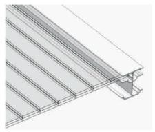
Place your next glazing bar into the polycarbonate sheet and push firmly into the channel. Please see diagram below. Fix the glazing bar onto the wall plate and gutter section, as previously described in step 8 make sure all glazing bars have a bead of sealer down both edges of the glazing bar to prevent water ingress as described above.
