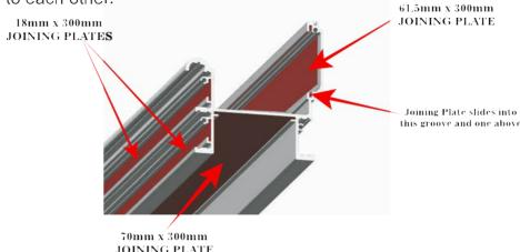
6. The two parts of the gutter must then be married together with no gap and the sudaflex allowed to set.
